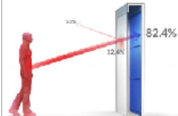
Fig. 1. Schematic of a Cold Tube radiant cooling panel (Dewell and Tamm, 2019). Heat transfer through the 18-gauge stainless steel membrane (Morrow).
