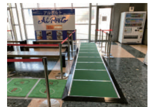
Vibration power generation
