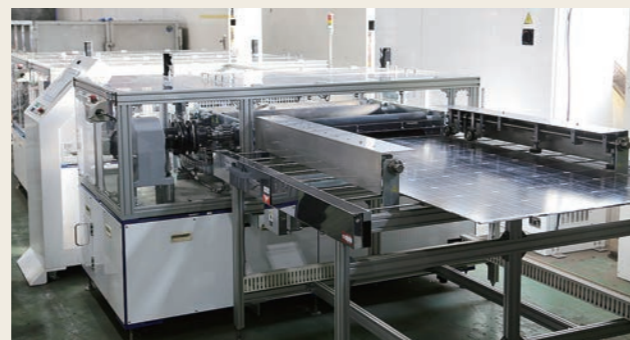
Machine to separate cover glass and photovoltaic cells of a solar panel Source: Hamada Co., Ltd.
