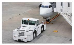
Fuel cell aircraft towing vehicle
