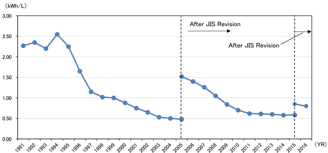
Figure 2-28 Progress of energy saving for electric refrigerators
