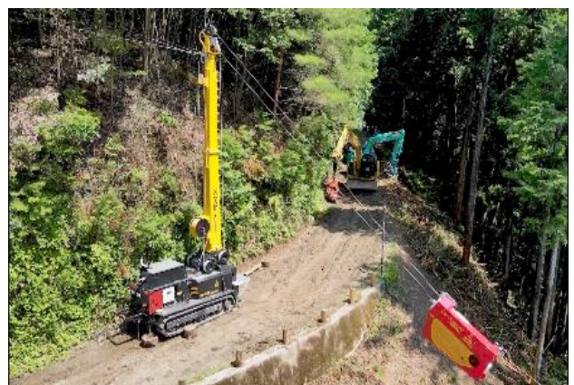
Advanced forestry machinery equipped with remote control function (Tower yarder)
