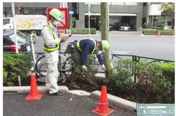
Inspecting street trees (checking tremors) (Confirmation of Steel rod penetration 2 )
