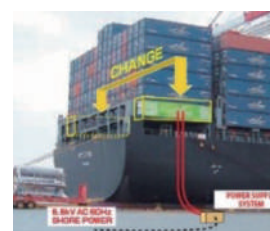
Alternative maritime power supply to ships at anchor
